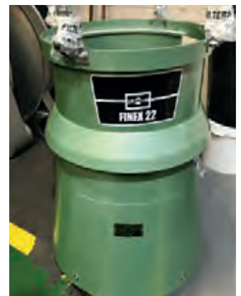
The refurbished sieve is now in situ...
