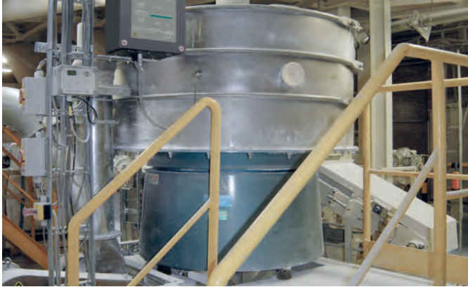
The new Vibrasonic Titanium Plus deblinding system will be demonstrated
