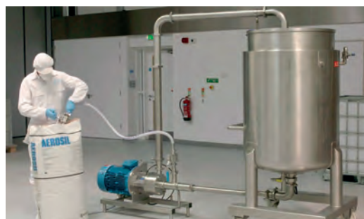
A powder feed wand attachment makes life easier for users
