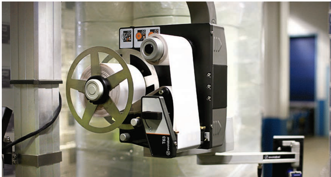
ILS's FlexWipe enables the pallet labelling of any dairy products that must be kept in sub-zero conditions
