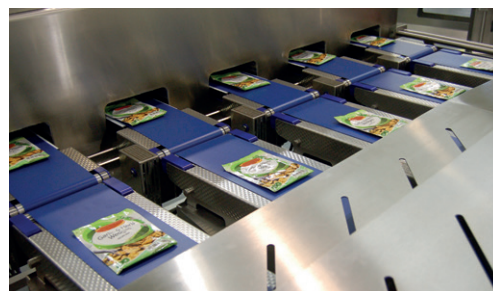
Multiple SG420 checkweighers in a manufacturing plant can be networked
