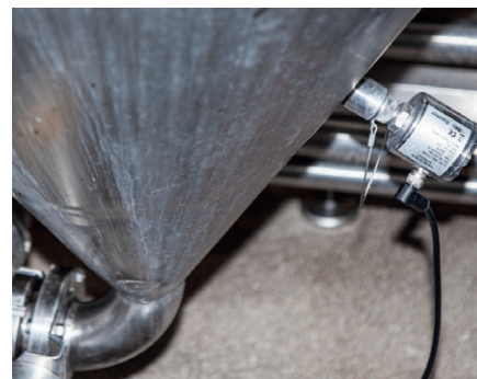
The sensors have a stainless steel housing
