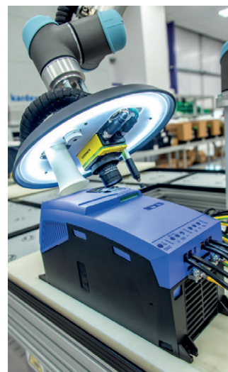
Working 16-hour shifts, the cobots inspect and test the range of devices
