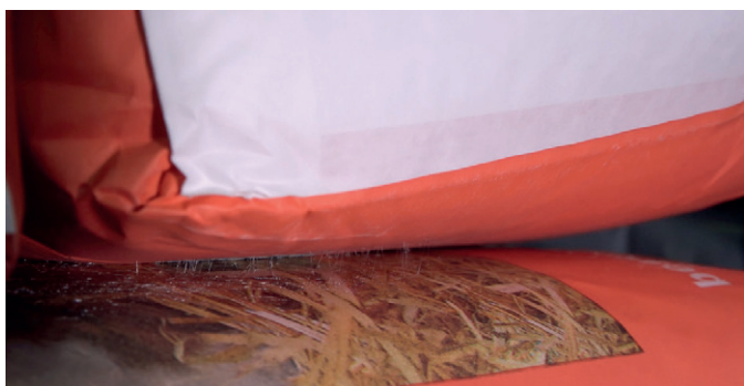
Adhesive is applied on both sides of the sack to allow an increase to ten layers
