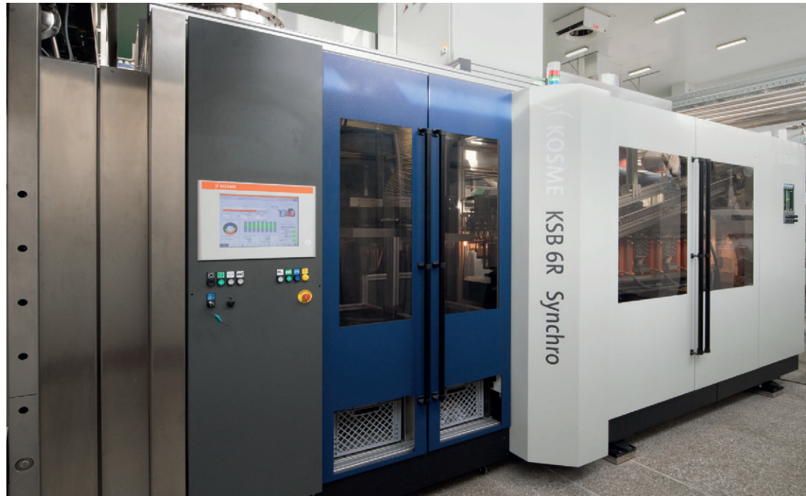
The PET-AseptBloc D aseptic block with H2O2 sterilisation consists of a stretch blow moulder, filler and capper
