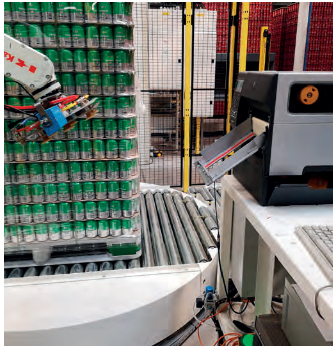
Kawasaki robots are used to apply labels direct onto the retaining straps
