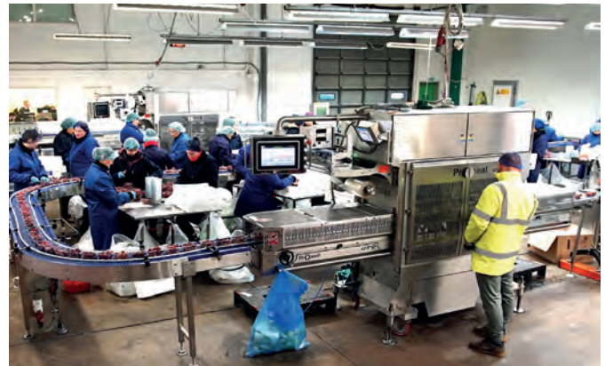
The conveyor is controlled and managed from the Proseal machine's interface
