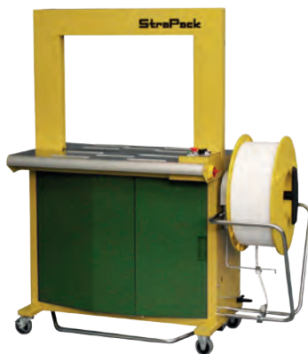
The SQ-800 features self-correcting technology to combat a short feed
