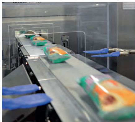
Final checks for foreign objects are carried out by x-ray systems and metal detectors at the bakery
