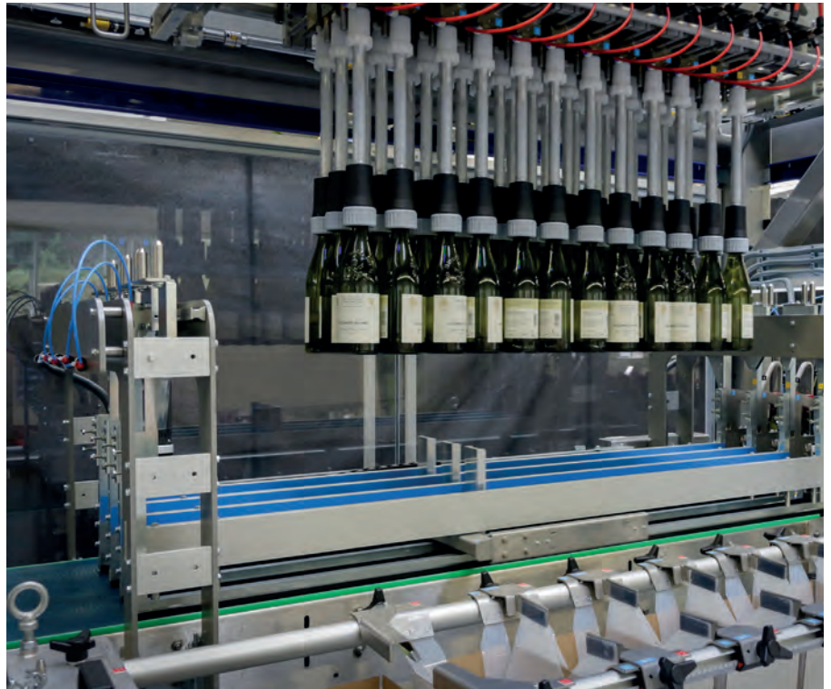
Flow and speed management at every step of the packing process protects glass bottles/labels
