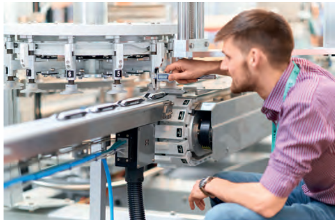
The 'paper-ON-form' retrofit kit for cold-sealable paper packaging allows for existing horizontal flow wrappers to be converted from plastic only materials
