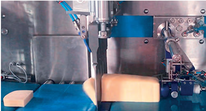
Several cheese types can be handled without the need to change any tooling
