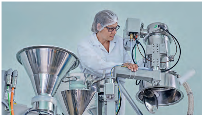
The vacuum conveyor is easy to clean which helps with product changeovers
