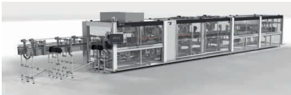
KHS's Innopack Kisters CNP machine handles cardboard can toppers from Smurfit Kappa and other manufacturers
