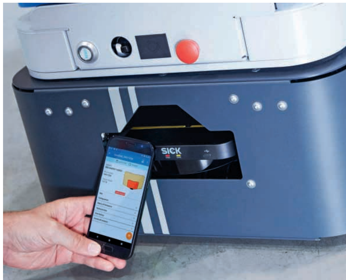
Sick's solid-state safety scanner is designed to boost productivity for small AMRs currently being adopted
