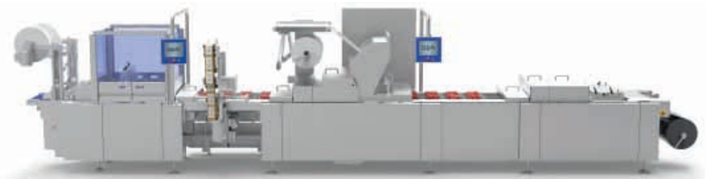
Quality enhancements have been achieved on the PowerPak SKIN.50 by the new top film guiding and pre-heating station
