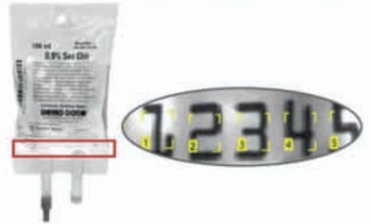
Verifies characters printed on reflective materials
