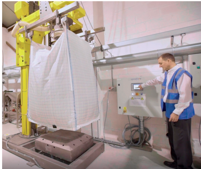
Spiroflow's bulk bag filler features a patented cone table densification system
