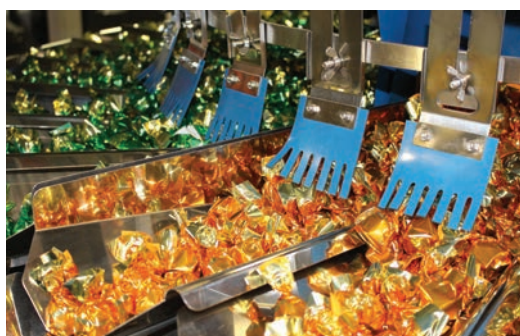
The 32 heads of the new weigher are divided into sections
