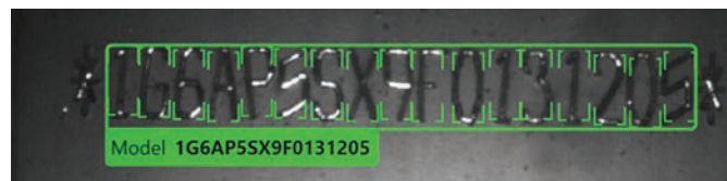
The Blue Read tool reliably deciphers and recognises skewed fonts and codes
