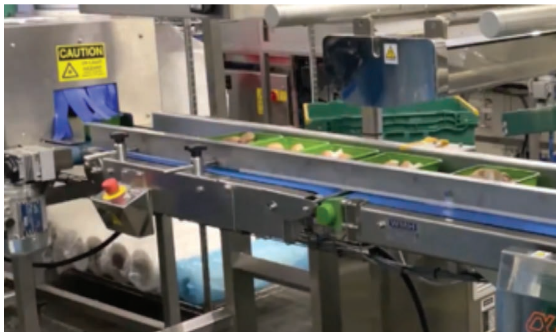
Belt speed is matched to film speed, so any mushrooms proud of a punnet remain in the punnet during packing
