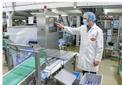
The Synus checkweigher in action at Sula
