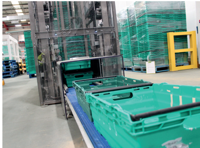
In operation, the new Dual Crate unit handles 16 to 18 crates per minute
