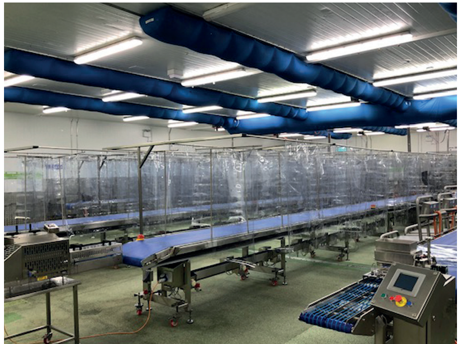
Protective screens with stainless steel frames and clear plastic sheeting are protecting workers
