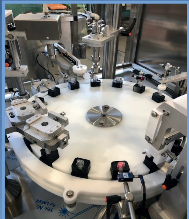
Omas Filling and Capping POD machine for E-liquid pods. Designed for quick easy change over between pods and flavours available as both semi-automatic and fully automatic high-speed lines.
