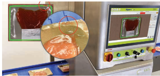
The seal inspection unit copes with paper-based backings
