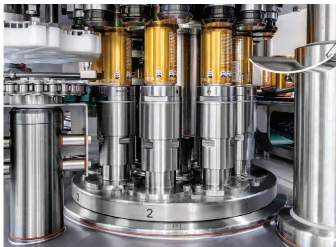
The seamer section is made entirely of stainless steel for added durability
